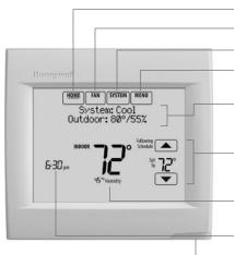
The screen lights when you press any button. It stays lit for 7 seconds after you complete changes. Depending on how your thermostat was installed, the screen light may always be on.
