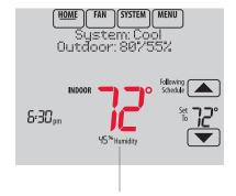
Temperature reading depends on location of sensor
